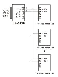
3. Half-duplex communication connections between UT-208 interfaces
