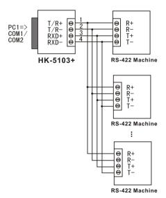
3. Half-duplex communication connections between HK-5103+ interfaces
