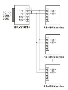
3. Half-duplex communication connections between HK-5103+ interfaces
