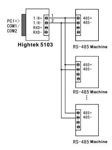
3. Half-duplex communication connections between Hightek 5103 interfaces
