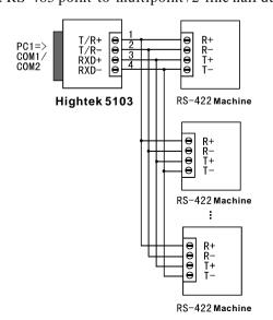
3. Half-duplex communication connections between Hightek 5103 interfaces
