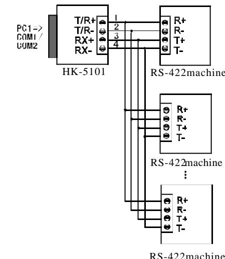
3.HK-5101 Full-duplex communication connection between interface converter
