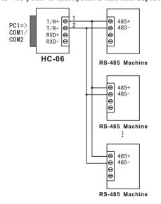
3. Half-duplex communication connections between HC-06 interfaces
