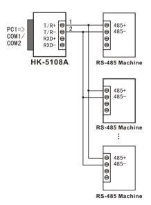
3. Half-duplex communication connections between HK-5108A interfaces
