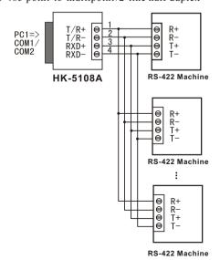
3. Half-duplex communication connections between HK-5108A interfaces
