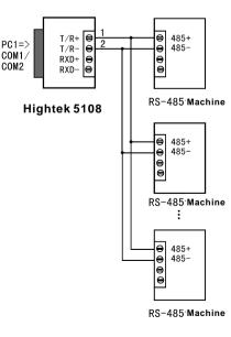
3. Half-duplex communication connections between Hightek 5108 interfaces
