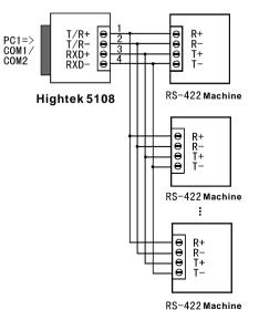
3. Half-duplex communication connections between Hightek 5108interfaces
