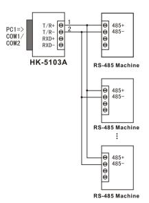
3. Half-duplex communication connections between HK-5103A interfaces
