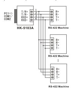
3. Half-duplex communication connections between HK-5103A interfaces
